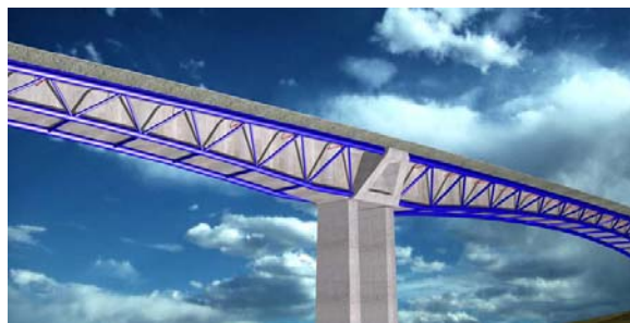
Fig. 4 Widening the deck using a steel truss partially connected to the existing deck
