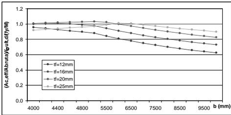
Figure 6a: Plate girder. Results depending on the width ( $b$ )
