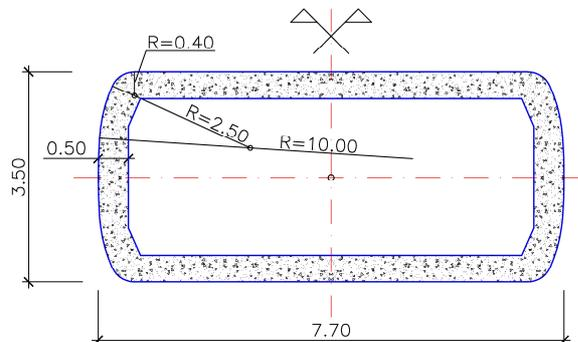
Fig 6. Cross section of the arch
