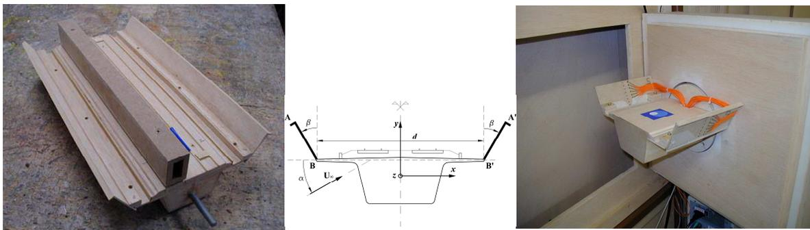
**Fig 16.** . Model of the deck, including wind protection barriers
