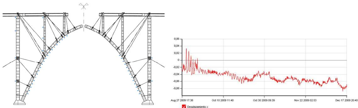
Fig 20. Results of the measurement of the movement of the central segment of the arch
