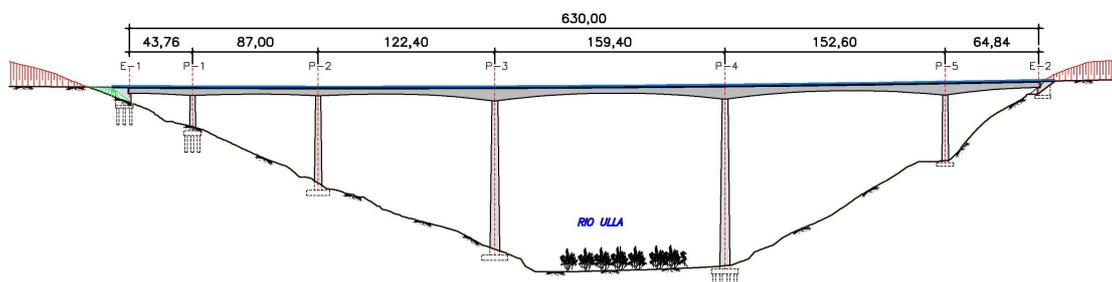
Fig 2. Solution 1. Segmental prestressed concrete bridge
