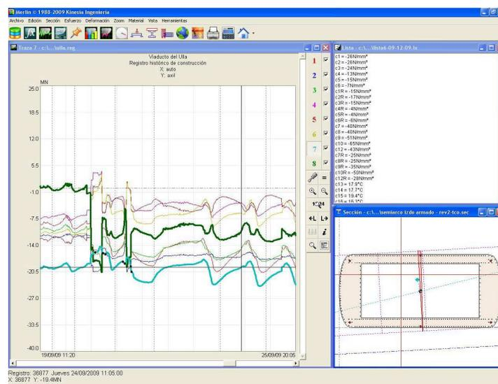
Fig 19. Results of the monitoring of the relevant cross section of pier P5
