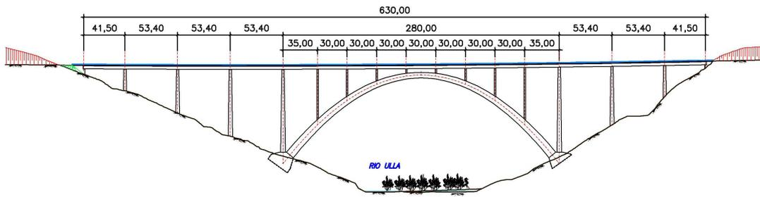
Fig 4. Solution III. Concrete arch (central span = 280 m)
