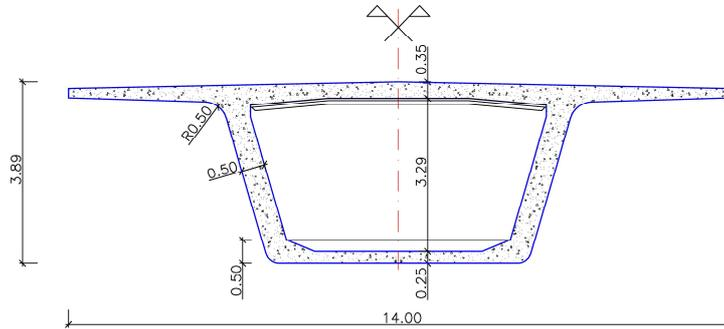
**Fig 9.** Cross section of the deck
