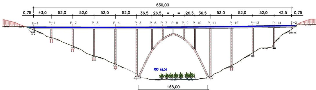
Fig 3. Solution II. “Ojival” arch (central span = 168 m)
