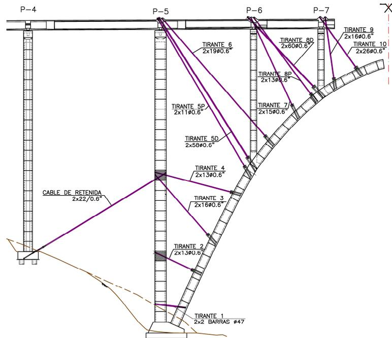
**Fig 13.** Structural scheme of the temporary ties for constructing the arch
